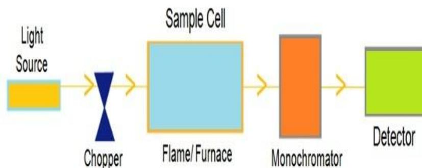
Fig. 3: Schematic Diagram of AAS (Csuros, M., Csuros, C., 2002)
